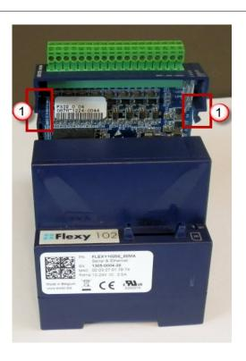
Hooks to be pressed are off-centered – press while pulling upwards
